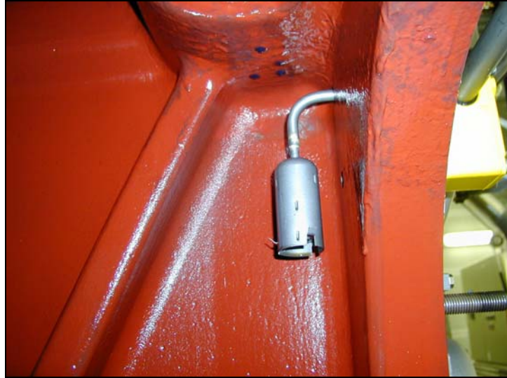
Fig. 6 & 7 : The suction funnels in these crankcase compartments will ensure an effective oil separation and permit the unobstructed oil mist transfer to the suction pipes of the OMD system. The suction funnel with the long cup design shown on the right (double labyrinth inside) has significantly improved the oil mist sampling and can be utilized in engines with CW or CCW crankshaft rotation.
