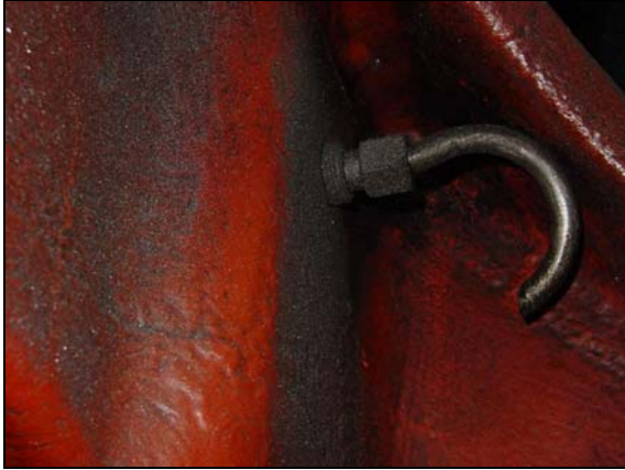
Fig. 1 & 2: Suction Elbow collects oil and clogs suction pipes. Consequences: Suction pipes and OMD become contaminated with oil, causing slow detector reaction and repeated false alarms.
