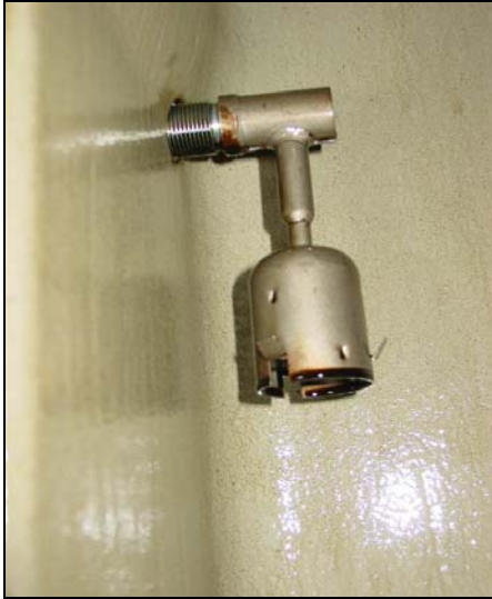
Fig. 6 & 7 : The suction funnels in these crankcase compartments will ensure an effective oil separation and permit the unobstructed oil mist transfer to the suction pipes of the OMD system. The suction funnel with the long cup design shown on the right (double labyrinth inside) has significantly improved the oil mist sampling and can be utilized in engines with CW or CCW crankshaft rotation.
