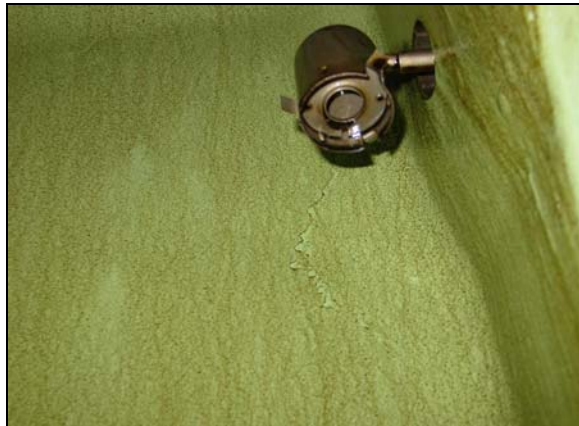
Fig. 5: Solution, install suction funnels. These separate the oil effectively and oil mist will reach the OMD fast and unhindered
